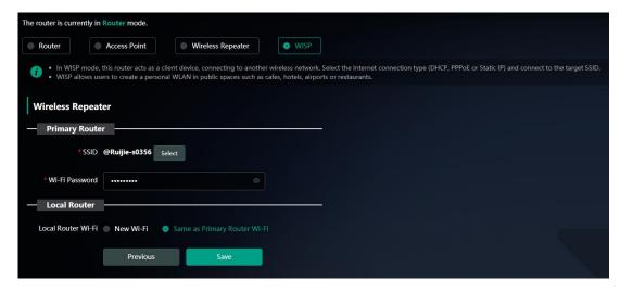
If you select New Wi-Fi, you can set a local SSID and password. Clients will search out a Wi-Fi signal different from the primary router Wi-Fi signal.
