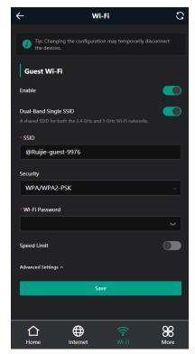
Dual-Band Single SSID: After this feature is enabled, the 2.4 GHz SSID will be consistent with the 5 GHz SSID and the 5 GHz band will be preferred. The 2.4 GHz signal is strong but easily interfered by various wireless signals. The 5 GHz band boasts fast speed, low latency and less interference.
