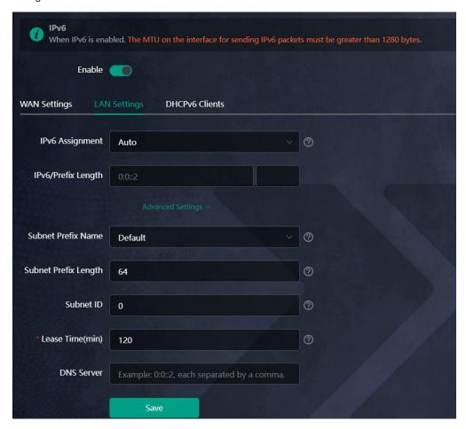
Click **DHCPv6 Clients** to view the list of clients that have obtained IPv6 from the router.
