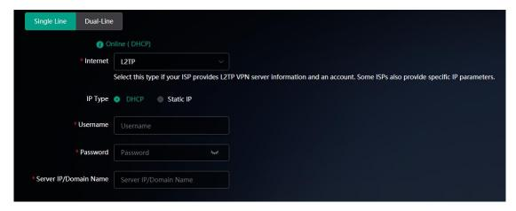
Static IP: In addition to the username, password, and server IP or domain name provided by the L2TP service provider, enter the static IP address assigned by the uplink device (like a modem), subnet mask, gateway IP address, and DNS server address for internet access, and click Next.
