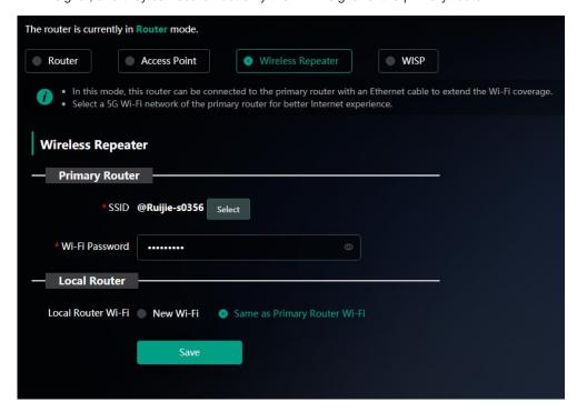
o If you select **New Wi-Fi**, you can set a local SSID and password. Clients will search out a Wi-Fi signal different from the primary router Wi-Fi signal.
