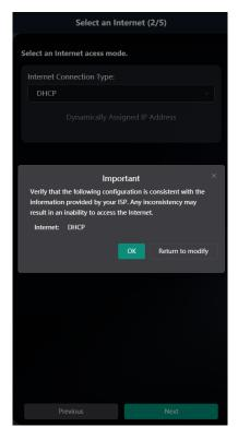
(3) Click **Next**. On the **Set Wi-Fi** page that opens, enter the Wi-Fi SSID and password and management password for the extender.
