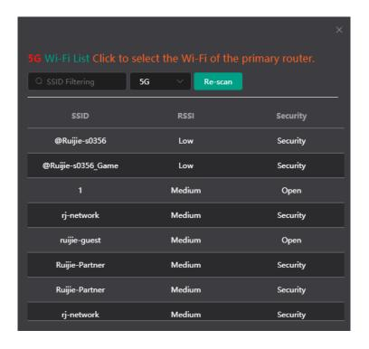
(2) Select the Wi-Fi network of the primary router to be relayed. The **Local Router** configuration item is displayed. If the primary router's Wi-Fi network is encrypted, enter the Wi-Fi password.
